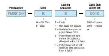
Example: Order number for a panel Black in color, loaded with 12 PSC adapters (2 six packs), connectors and a cable stub 10 meters in length.
