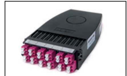
FC4U12LDMF, FX Ultra Cassette, OM4, 12 ports, MPO-12 (male), LC Duplex, Type-A, Erika Violet adapters
