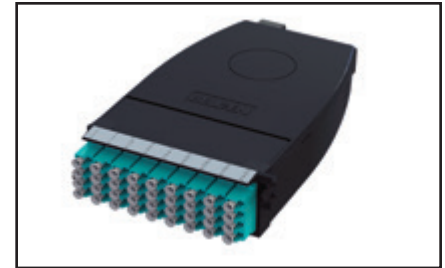
FC3H18LDMF, FX UHD Cassette, OM3, 18 ports, MPO-12 (male), LC Duplex, Type-A, Aqua adapters
