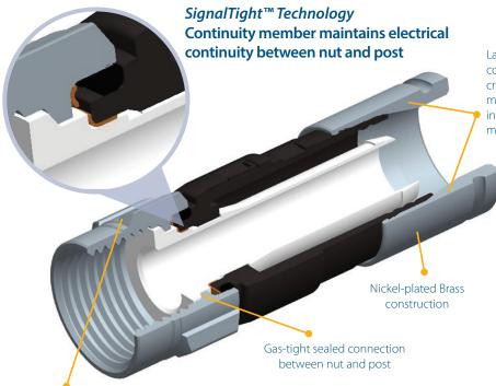
Innovative nut design provides 7/16 wrench capability for tech installation, while appearing to the subscriber as a finger-tightening fitting
