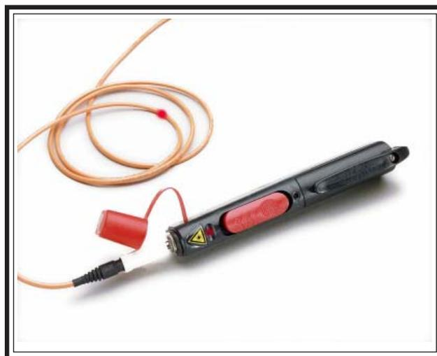
This single basic tool is one that all installers, and maintenance personnel should have in their tool kit. It is the most economical test tool for quickly verifying continuity, checking the validity of patch cables before or after installation, test and find breaks in LANs, verifying short lengths of installed fiber, or looking for cracked fiber in splice cases, bad connectors, tight crimps in fiber cable, backbone breaks or anywhere light continuity needs checking.
