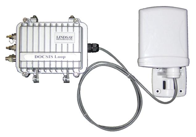
The DOCSIS Gateway allows the use of any low voltage Access Point on the HFC strand. You can use Lindsay recommended Mikrotik Access Points or Access Points from Ubiquiti, Compex, Alcon, etc. You can use any AP that accepts 12Vdc passive POE (4,6+, 7,8-) and that does not require more than 8 Watts. Other IP devices that meet the voltage and power requirements, like IP cameras, can also be used.
