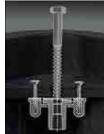
Non-Seizing Bolt System Allows Field Replacement
