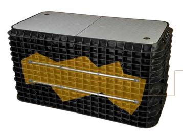
Stainless steel tube is constructed into sidewall of pit to prevent sidewall deflection on BULK bodies 18" (457 mm) and deeper.
