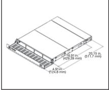
FX UHD 1U Housing with mounted Splice Housing Kit
