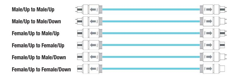
Achieve the most accurate link test measurements with any test equipment. Whether test equipment has a male or female interface, the PanMPO<sup>™</sup> Connector can be configured to fit, without introducing a third test cord. This eliminates an added layer of variability, reduces errors and improves accuracy.
